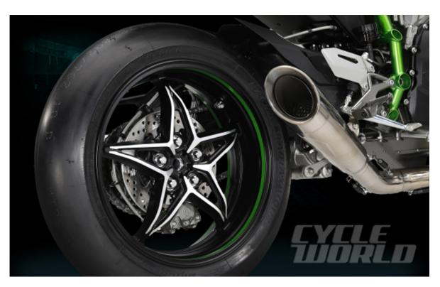
New five-spoke star-design wheels are finished in black and polished aluminum. As you'd expect on such a machine, the inner faces of the rim flanges on the H2R are knurled to prevent tire slip. The closed-circuit, non-DOT bike is delivered with 120/600R-17 and 190/650R-17 Bridgestone slicks. For the A-spec road-legal bike, tires are Bridgestone Battlax RS10SG.
