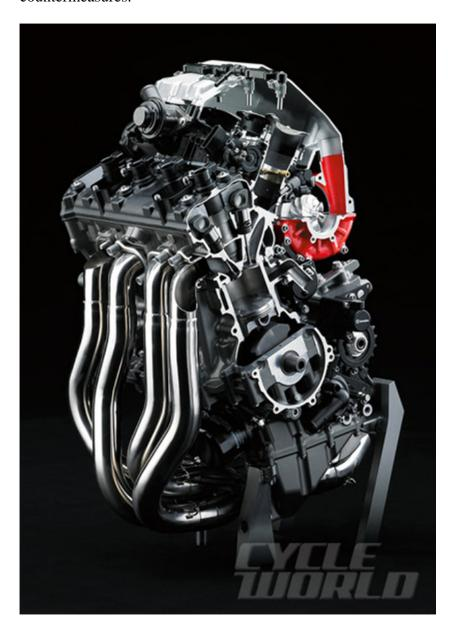
Power goes to a high-mounted hydraulically operated clutch on the right side with 5.5-inch-diameter plates—10 in the B-spec closed-circuit engine and nine in the A-spec. To keep plates free, the basket is treated with "Kashima coating," which combines the hardness of aluminum oxide ceramic with the low friction of the solid lubricant molybdenum disulfide. This is a slipper clutch, and, combined with KEBC engine-braking control, sliding or hop of the rear wheel during braking is prevented.
