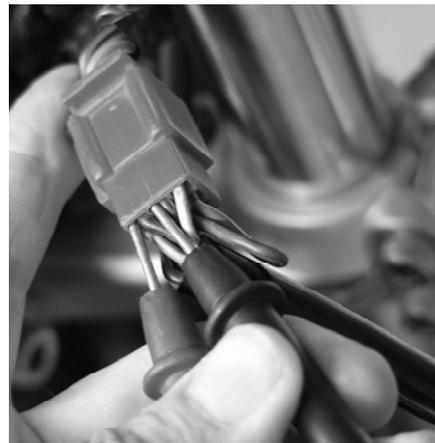
**Confirm the trouble spot by straddling it with the multimeter probes.**
