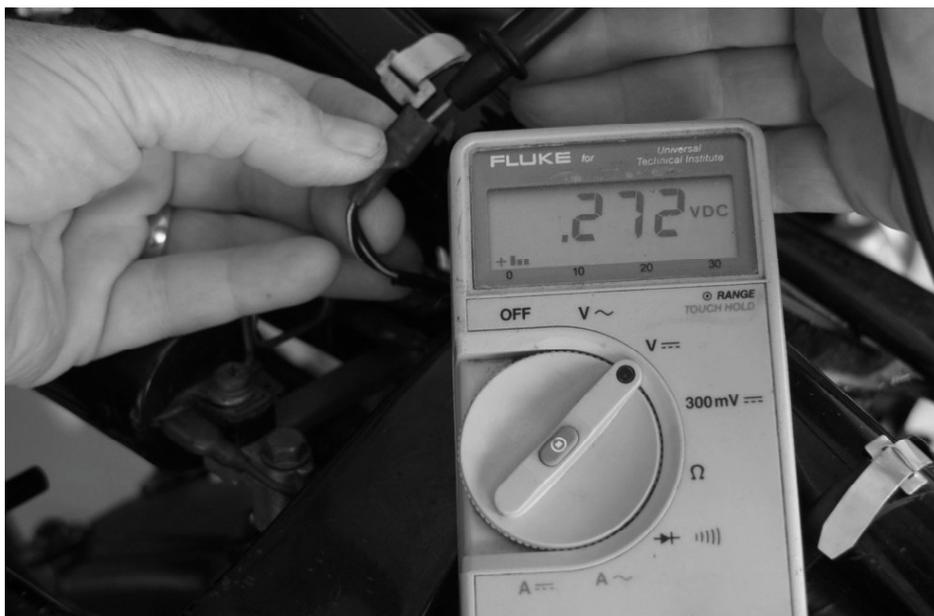
**The voltage drop test can uncover resistances too small for an ohmmeter to measure.**
