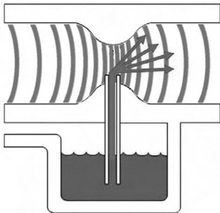
**Proportional changes in venturi air pressure draw corresponding splashes of fuel into the airstream.**
