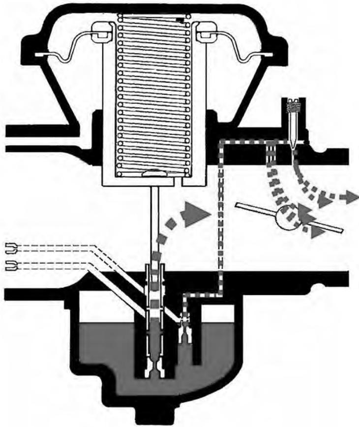
**The carburetor's various jet circuits help atomize the fuel, but cannot compensate for any change from baseline conditions.**
